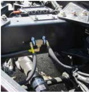
Chassis line Tee out to tyres note rubber hose sheathe
