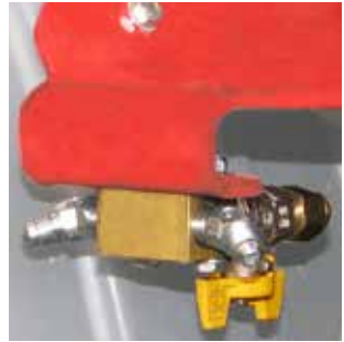
Feed hose Tee Block between wheels TA37004
