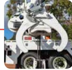
High torque, variable speed auger motor suitable for up to 900mm augers
