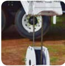
16mm non rotating hoist rope, with anti two block interlock and grooved drum for longer rope life
